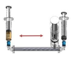
Begin the **Micro-Filtration** process by injecting the plasma back and forth through the 12mL syringes until the plasma retentate reaches 7mL or the desired amount.
