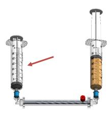
Remove the filter and attach the transfer syringe.
