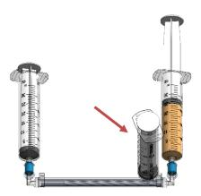
Break the seal of the effluent syringe, remove the red cap and attach the syringe to the effluent port.
