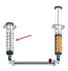
Remove the filter and attach the 30mL transfer syringe.
