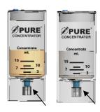
IMPORTANT!! MAKE SURE CLEAR CAP IS PLACED ON BOTTOM PORT PRIOR TO CENTRIFUGATION!!!
