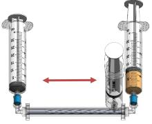
Begin the **Macro-Filtration** process by injecting the plasma back and forth through the syringes until the plasma retentate reaches approximately 10mL.
