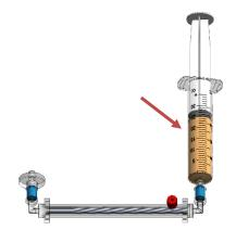
Remove the red cap on the near side of the effluent port and attach the plasma syringe.
