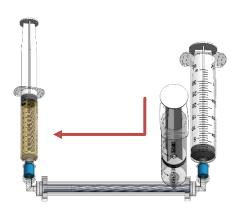
Inject the 10mL plasma retentate into the 12mL syringe
