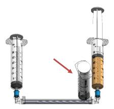
Break the seal of the effluent syringe, remove the red cap and attach the syringe to the effluent port.
