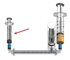
Replace the empty 30mL syringe with a 12mL syringe.
