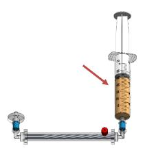
Remove the red cap on the near side of the effluent port and attach the 30mL plasma syringe.
