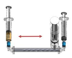
Begin the **Micro-Filtration** process by injecting the plasma back and forth through the 12mL syringes until the plasma retentate reaches 5mL.
