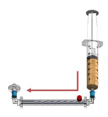
Inject plasma through the device until it reaches the filter.
