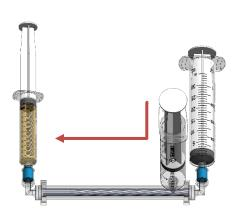
Inject the 10mL plasma retentate into the 12mL syringe
