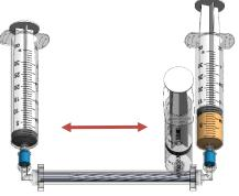
Begin the **Macro-Filtration** process by injecting the plasma back and forth through the 30mL syringes until the plasma retentate reaches approximately 10mL.
