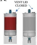
Close VENT LID and counterbalance device with equal volume.
