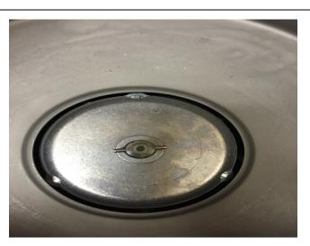
5. Take the rotor key and tighten the rotor nut by turning it clockwise until it is securely tight.
