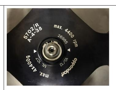
2. The triangles indicate the direction of the groove on the underside of the rotor.
